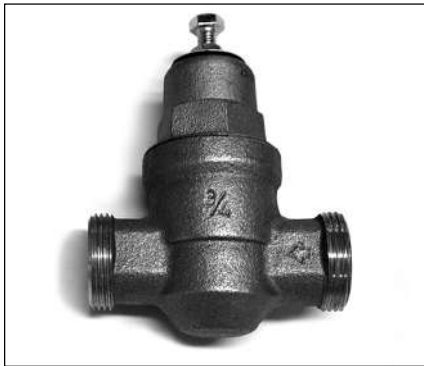
Figure 27 - A Pressure Reducing Valve is required if your home's water pressure is above 80 psi.
