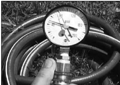
Figure 12 - Use a Water Pressure Gauge to make sure your home's water pressure is not too high.
