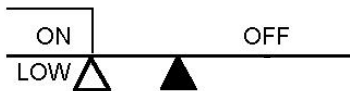
Figure 4-4 Lower Limit Deviation Alarm (Alarm Code 02, Alarm release in the first alarming situation)
