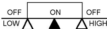
Figure 4-9 Deviation Band Alarm (Alarm Code 14, No alarm release in the first alarming situation)
