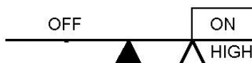
Figure 4-3 Upper Limit Deviation Alarm (Alarm Code 11, No alarm release in the first alarming situation)
