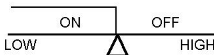
Figure 4-13 Absolute Lower Limit Alarm (Alarm Code 06, Alarm release in the first alarming situation)
